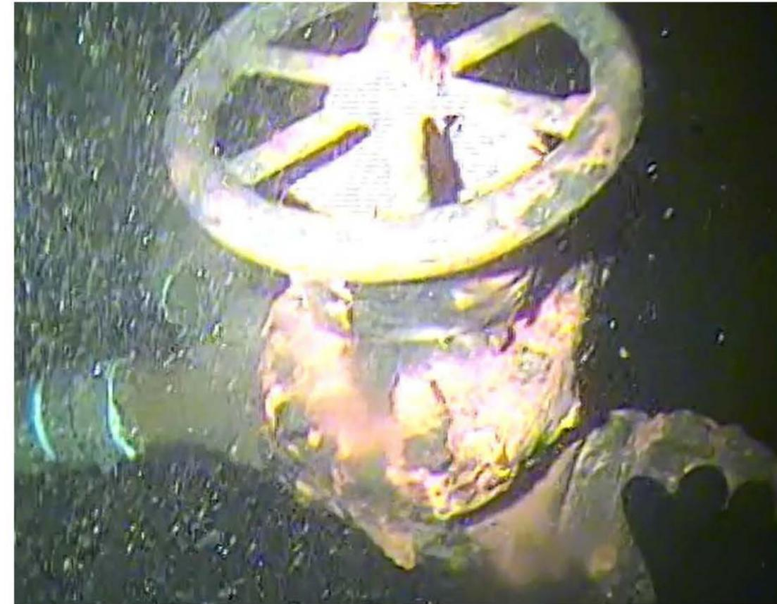
Photo # D3 – Corrosion at valve at wash line from diver's video
